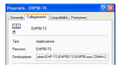
In some operating system the Destination field is enclosed in double quotation marks ("); in this case, the command COMM=N, preceded by a space must be outside as in the example below;
