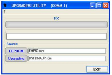
To start the process simply switch EHP-50C on and wait (few minutes) until the automatic transfer is completed.
